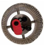
The **miniCTD probe** is a small and lightweight, budget-priced system designed for in-situ acquisition of scientific data in oceanic, estuarine and fresh water environments.
