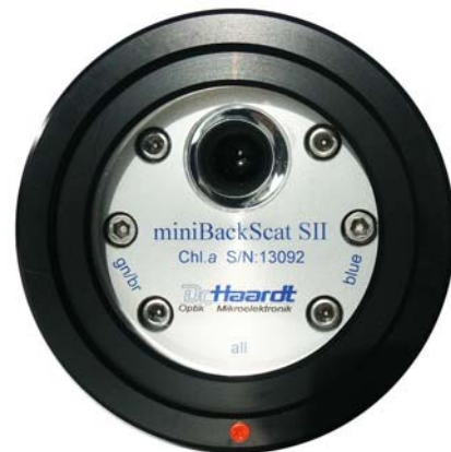
The front cap can be turned to select the group of algae to be detected.
