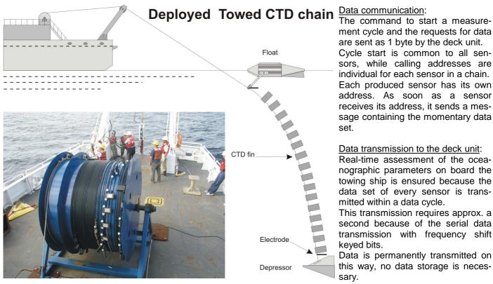
ment cycle and the requests for data are sent as 1 byte by the deck unit. Cycle start is common to all sensors, while calling addresses are individual for each sensor in a chain. Each produced sensor has its own address. As soon as a sensor receives its address, it sends a message containing the momentary data set.
